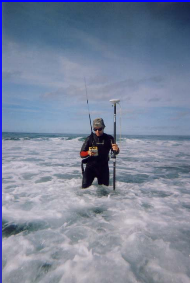
DGPS Trimble 5700 (vertical accuracy 5 cm)
